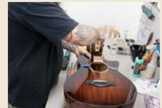
The removal of a Taylor neck is easy enough that the strings can simply be loosened to adjust the angle.
