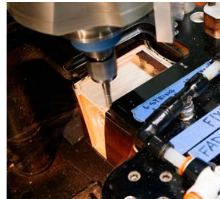
A CNC router cuts a precise pocket in a guitar body
