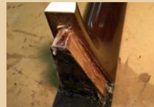
A view of a dovetail neck with some of the residual glue visible after it has been removed. Wood will need to be shaved from some locations of the dovetail and added to other locations in order to adjust the angle.
