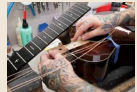
One of the precision-milled pocket spacers is swapped for another with a different micro-tapered thickness to alter the angle.
