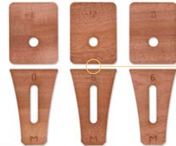
Neck Angle Spacers Laser-cut and milled in varying increments of .002 inch, these form the basis of setting the perfect neck angle. The spacers are inset (without glue) into the two pockets where the neck will meet the body and can be changed easily to micro-calibrate the neck angle in Final Assembly and throughout the guitar's life.
