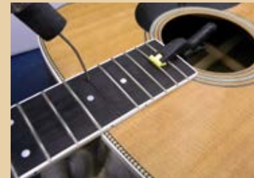
After a fret has been removed, steam is channeled through the fret slot into the dovetail neck joint to soften and loosen the glue.
