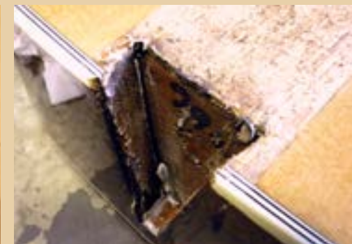
A view of the dovetail mortise and residual glue after the neck has been removed.
