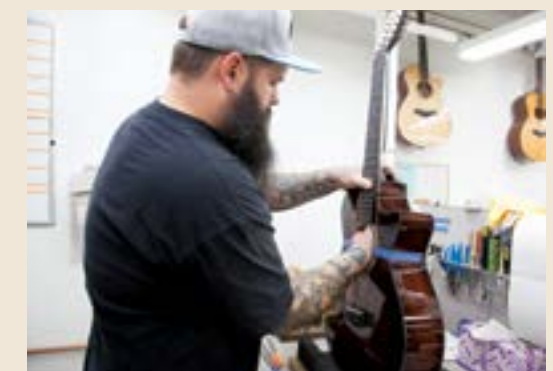
The neck is easily reattached through the soundhole using a secure three-bolt assembly.
