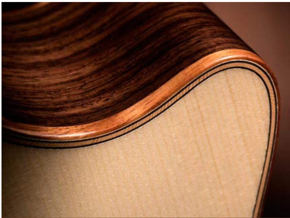
Top: Three-ring rosette featuring bias-cut, Herringbone-style Douglas fir strips with maple and black trim; Above: Non-figured koa binding with top edge trim of bias-cut Douglas fir, black and maple; Right: The new weathered brown pickguard. Opposite Page (top down): "Reflections" fretboard inlay; A non-figured koa back strip matches the binding
