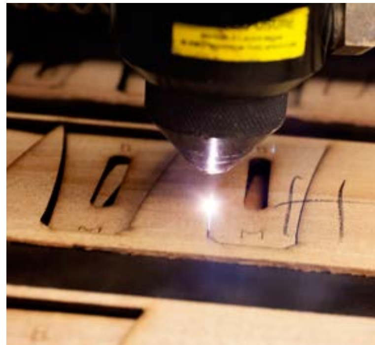
Top down: The neck heel is shaped on a CNC mill; neck angle spacers being laser cut
