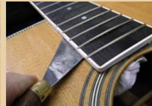
A flat bridge/fingerboard removal knife is used to separate the fretboard extension from the top.
