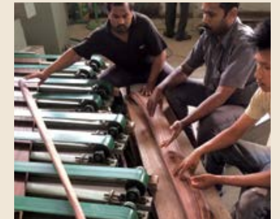
Top down: (L-R) Taylor's Chris Cosgrove, Lak, Dev and Mahadev Gopalakrishnan, and Taylor's Charlie Redden at the Gemwood mill; a rosewood log is cut into slabs; freshly sliced sheets of rosewood veneer are held flat before being put through a dryer to flatten them permanently
